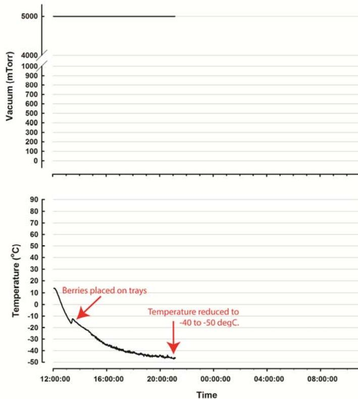
Firstly, the pepperberries are placed onto trays, a single layer thick, and then deep frozen to between  $-40^{\circ}\text{C}$  and  $-50^{\circ}\text{C}$ .
