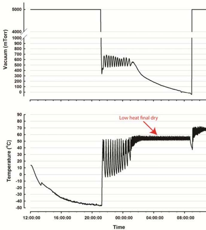
Thirdly, the final bound water is removed by continuous low heating of the trays.
