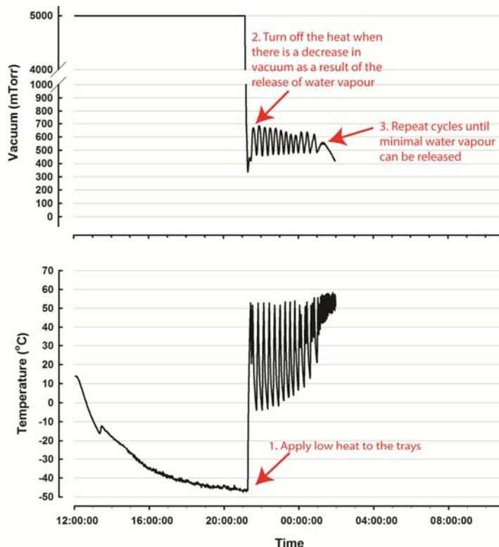
Secondly, once fully deep frozen, the vacuum pump removes the air from the chamber. When the pressure in the chamber reaches 0.066 kPa (500 mTorr), the trays are then gently heated (typically to around a maximum of  $52^{\circ}\text{C}$ ).
